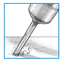
Typically the solid form is applied to the tool before start-up. In a block form, it can hand held and a drill bit can be touched to the block before drilling or the block may be swiped across the surface to be drilled. Only a minimal amount is required when drilling through thin material.
