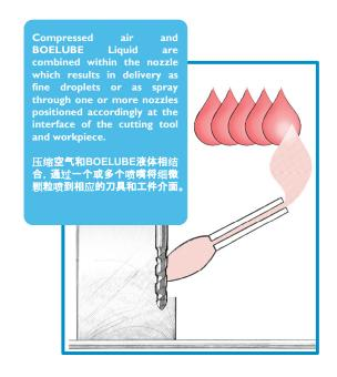
Milling produces machined surfaces by removing metal or other material using a rotating cutter having a certain number of cutting elements or teeth. A characteristic feature of the milling process is that each tooth of the rotating cutter takes a portion of material in the form of small, individual chips.
